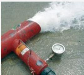
Flow test on systems indicate losses in hydraulic calculations due to build up in pipes caused by MIC Bacteria. "We've had great success eliminating the system leaks and odors in water"
