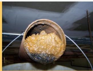
**#3- Slime forming Bacteria** add to the blockage of water through the system. SFB are known to begin the MIC bacterial consortium. Our Biocides eliminate 99-100% of bacteria in 3 hours.
